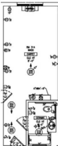
Level A: Full Survey of Model Room with Electrical Finish
